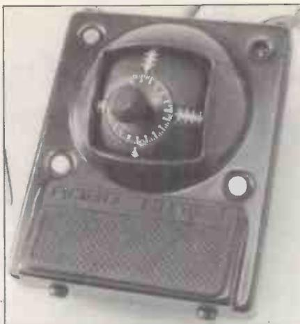
The Bit Stik controller includes three buttons as well as the joystick; a power-on light occupies the top-right position.
